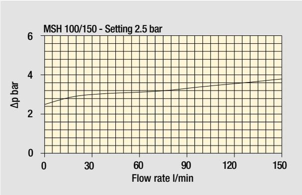
The curves are plotted using mineral oil with density of 0.86 kg/dm<sup>3</sup> in compliance with ISO 3968. Δp varies proportionally with density.
