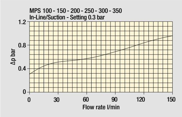
The curves are plotted using mineral oil with density of 0.86 kg/dm<sup>3</sup> in compliance with ISO 3968.
