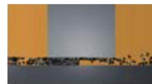
Solid contamination mainly causes surface damage and component wear.
