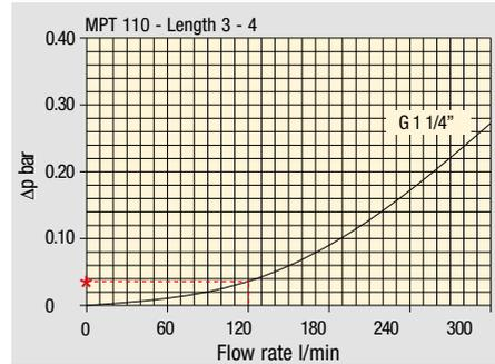
Filter housings Δp pressure drop. The curves are plotted using mineral oil with density of 0.86 kg/dm³ in compliance with ISO 3968. Δp varies proportionally with density.
