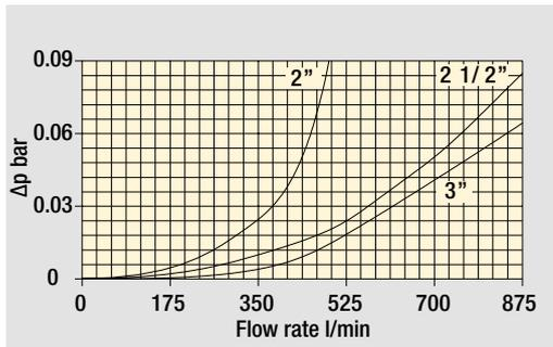
The curves are plotted using mineral oil with density of  $0.86 \text{ kg/dm}^3$  in compliance with ISO 3968.
