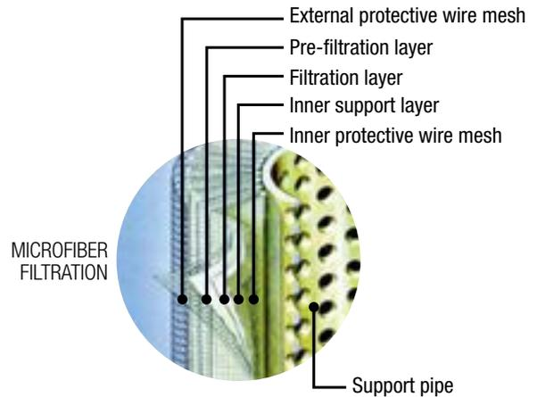
The filtration efficiency of metallic mesh filtrations is defined as the maximum particle size that can pass through the meshes of the filtering grid. The efficiency of microfibre and paper filtration ( $\beta_{x(c)}$ ) is defined through a lab test called Multipass Test. The efficiency value ( $\beta_{x(c)}$ ) is defined as the ratio between the number of particles of certain dimensions detected upstream and downstream of the filter.
