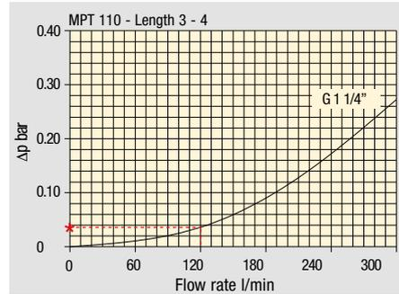
Filter housings  $\Delta p$  pressure drop. The curves are plotted using mineral oil with density of  $0.86 kg/dm^3$  in compliance with ISO 3968.  $\Delta p$  varies proportionally with density.
