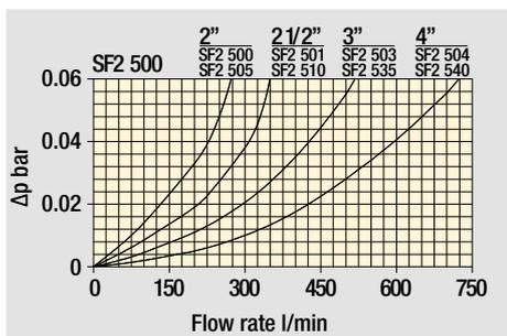
Filter element  $\Delta p$  pressure drop
